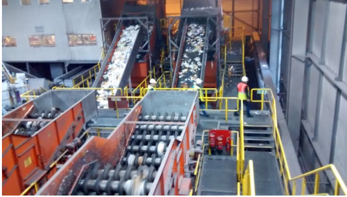
Figure 4: Bywaters MRF paper and cardboard sorting machinery
